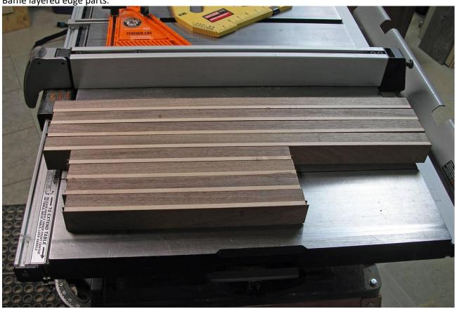
Gluing up baffle edge detail picture frame.
