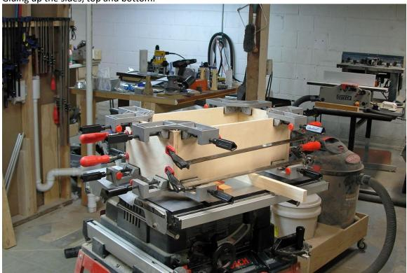
Adding  $\frac{1}{4}$ " firring strips to  $\frac{1}{2}$ " thick side walls.
