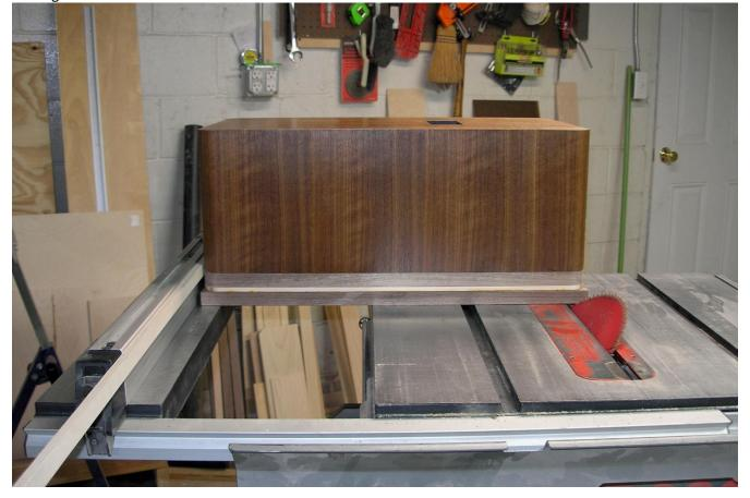
Box with 45-degree bevels cut. Oops, the biscuits used to join the two-piece walnut baffle are exposed. Time to learn how to do inlays.
