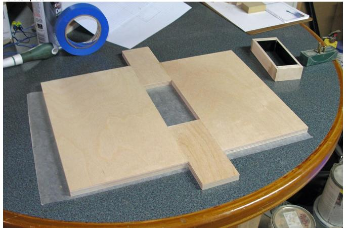
Cutting port cut out with a top bearing bit.
