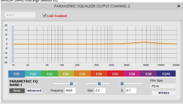
MiniDSP 2x4HD 1M 1Khz woofer LP and midrange tweeter HP. Gated measurement good down to 250Hz.
