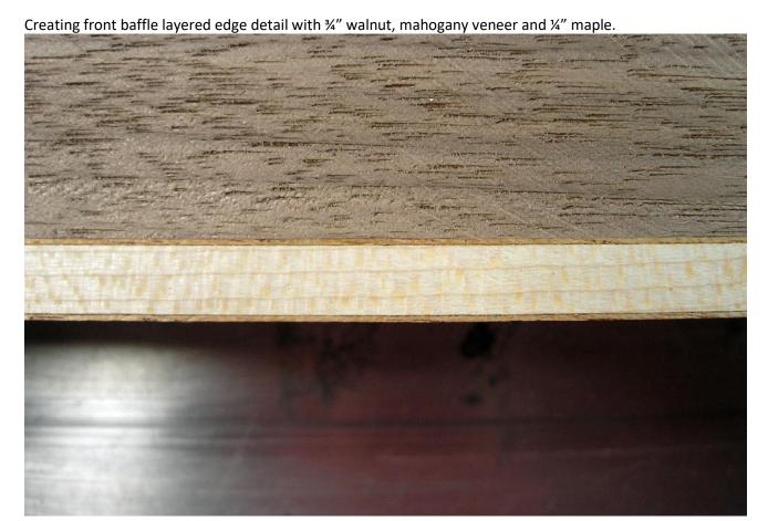
Baffle layered edge parts.
