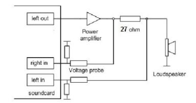
Figure 3.2 General measurement setup for loudspeaker impedance measurements
