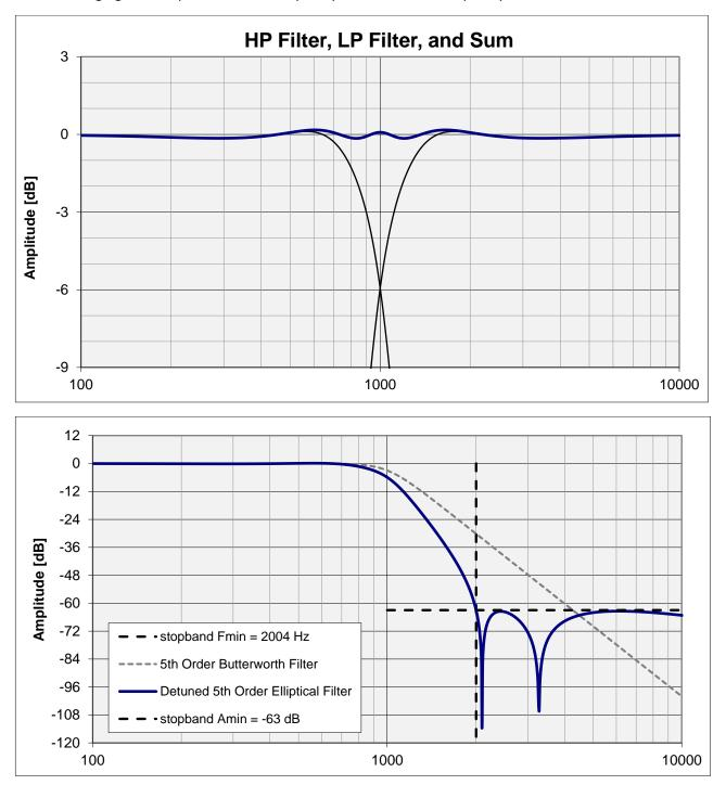
The following figures are plotted versus frequency for a crossover frequency of 1k Hz.
