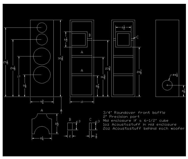
Here is a picture of the internal construction, to help give an idea of how things go together. The two shelf braces do not necessarily need to be shaped like these – just be sure there is a similar shape:
