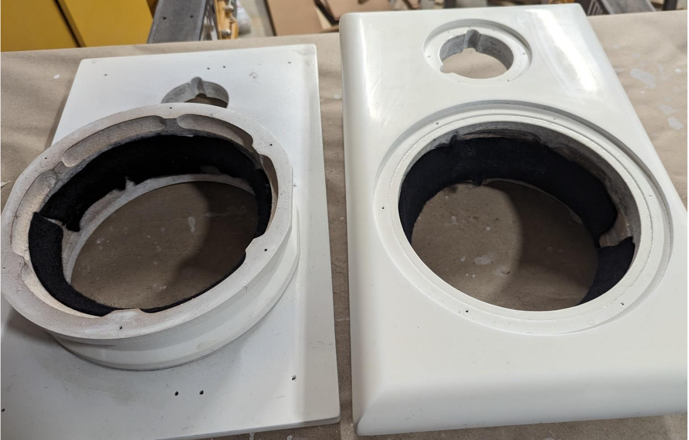
Figure 4: Isobaric chambers - inside lined with 1/4" wool felt
