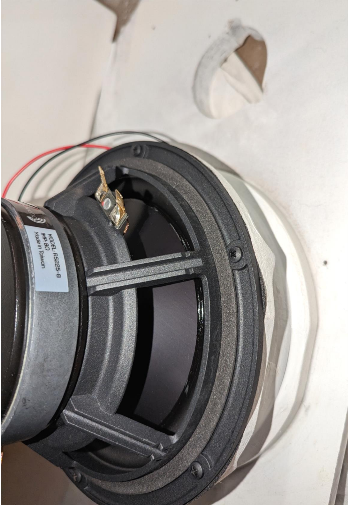
Figure 6: Inside/rear-woofer attached to isobaric tunnel (the light & shadows are playing some weird tricks here)
