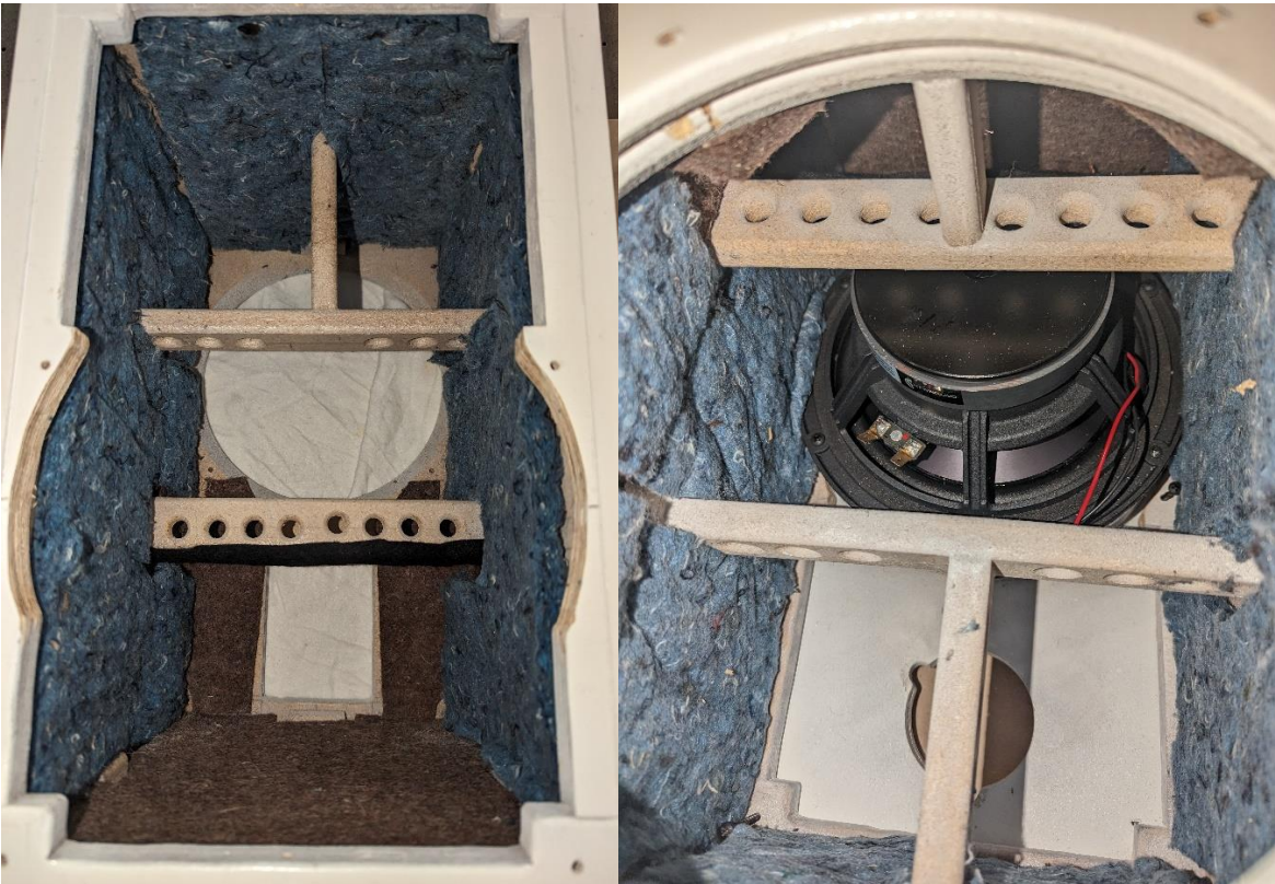
Figure 10: Cotton/recycled denim insulation, front baffle with isobaric tunnel and driver attached
