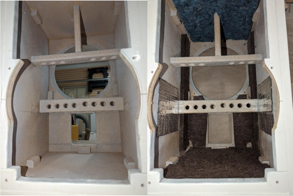
Figure 10: Cotton/recycled denim insulation, front baffle with isobaric tunnel and driver attached
