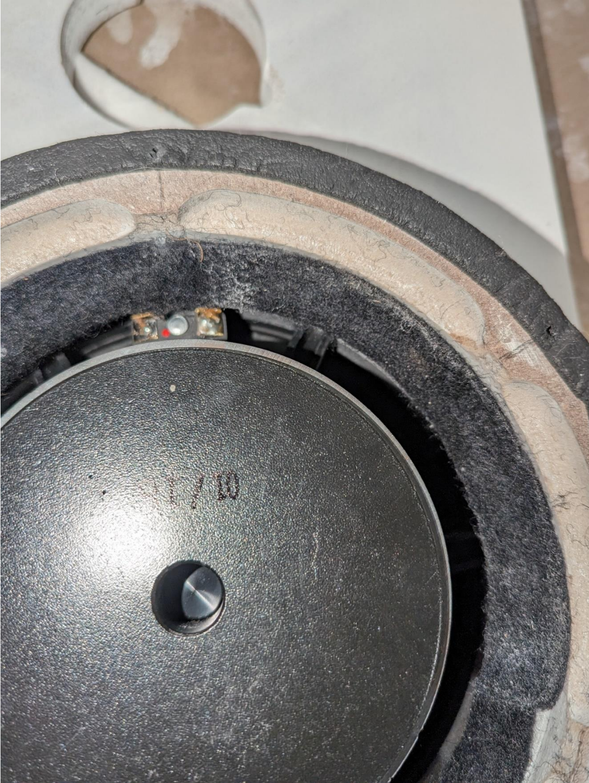
Figure 5: Isobaric tunnel - rear view with front woofer installed on baffle 3
