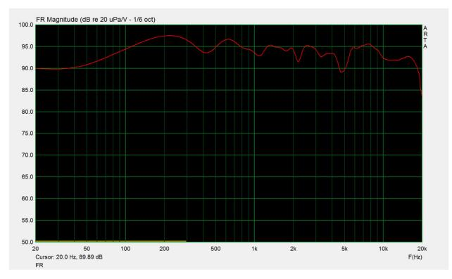
A very slight downward spectral tilt. The 5db dip at 5k will disappear off-axis. The 2.1k dip disappears off axis, as well. All in all – not bad at all for the price of the drivers.
