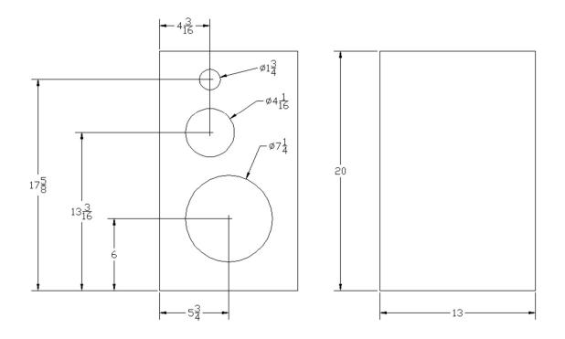
The four 18-1/2" panels serve as front, rear, and side baffles. Be sure that the top and bottom are glued to the top and bottom of the side panels, and that the front and rear are the narrow sides. If glued up correctly, the dimensions will match above so be sure to think it through first. Use scraps as braces, I ran one left to right and a couple angle braces here and there. What's important is that each panel is tied to at least one additional panel and all will be well.
